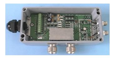
The sensor electronics enclosure is rated to IP65/NEMA 4, -20 to 70C and designed to EEx ib e (CENELEC & FM) hazardous environment safety standards.
